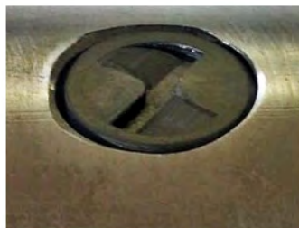
Close-up of an Screw Tag mounted into a pipe; notice that the tag is mounted flush to the surface of the pipe. Recessing the tag into the pipe deeper than shown may adversely affect the ability to interrogate the tag.
