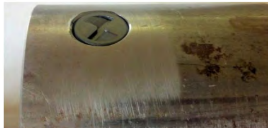
Close-up of an Screw Tag mounted into a pipe; notice that the tag is mounted flush to the surface of the pipe. Recessing the tag into the pipe deeper than shown may adversely affect the ability to interrogate the tag.
