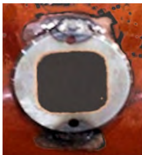
Correctly welded "spot" welds
