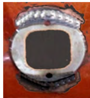
Incorrectly welded - too far around tag
