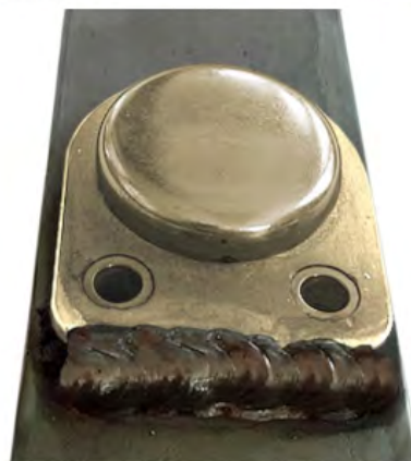
Correctly welded across the end of the tab
